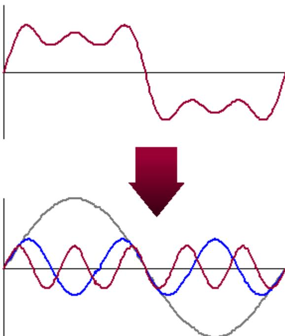
Figure 5: Distorted Wave Composed by the Superposition of a 50 Hz Fundamental and Smaller Third Harmonic and Fifth Harmonics.
